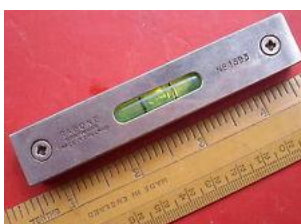
The picture shows a spirit level placed against a scale edge
